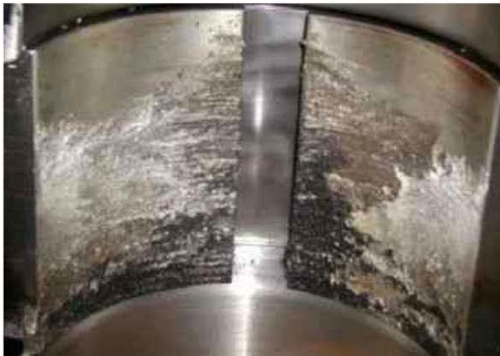
Figure 27 — Coloured surface due to loss of lubricant, melting out, seizure (material: steel/tin-based white metal)
