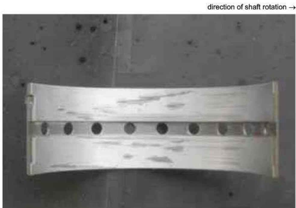
Figure 36 — Chevron-like defect caused by particles from iron nitride compound layer of nitrided shafts (material: steel/lead bronze/electroplated overlay)
