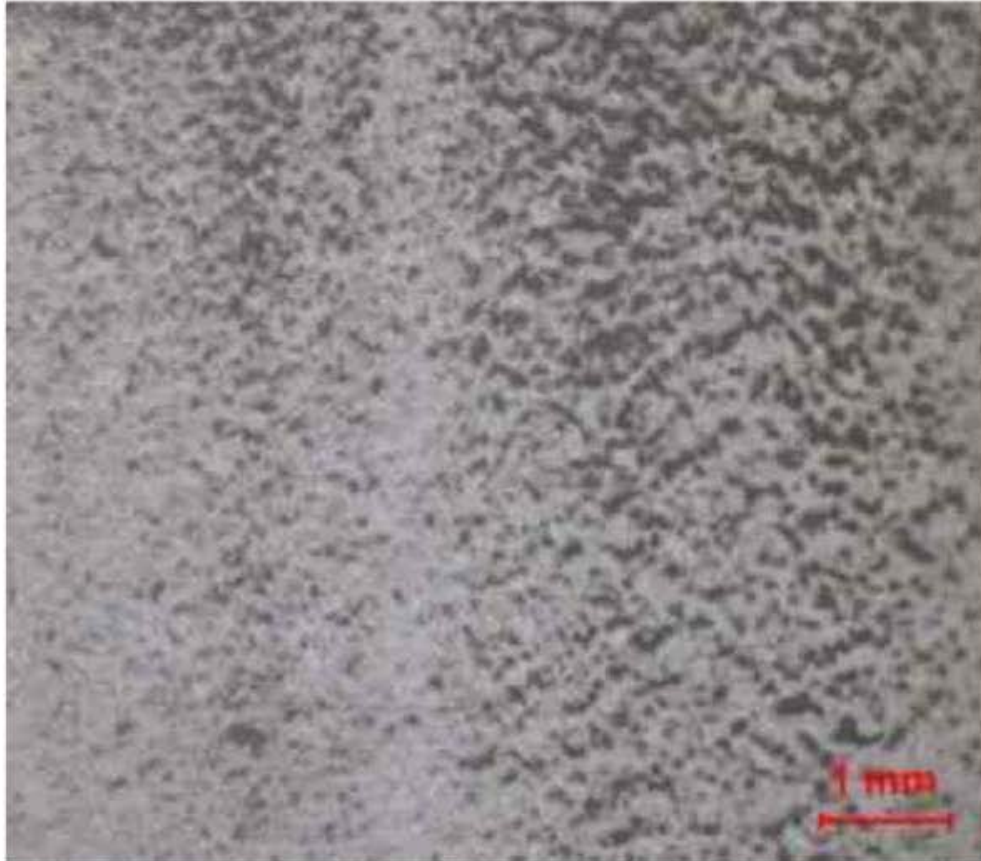
Figure 42 — Deposit of oil carbon on galvanic surface
