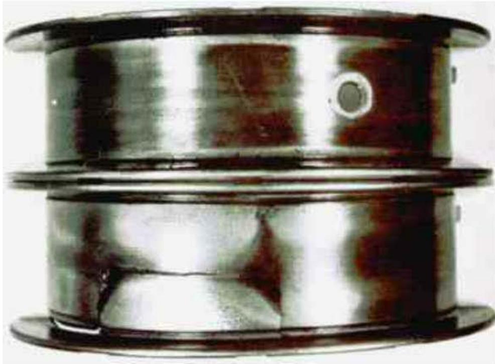
Figure 53 — Fracture of the steel backing (commencing at the top in an axial direction within an area exhibiting pronounced signs of movement, progressing circumferentially and finally deviating towards the flange)
