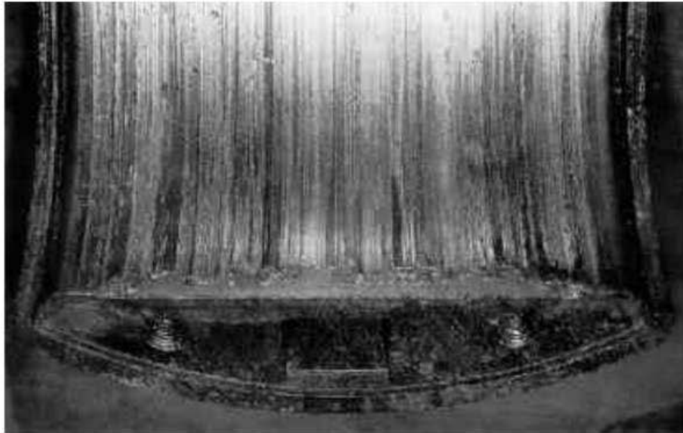
Figure 32 — Cement mill bearing with contamination by cement particles entrained by the oil as a result of damaged seals. Particle-migration tracks are visible (material: steel/tin-based white metal)
