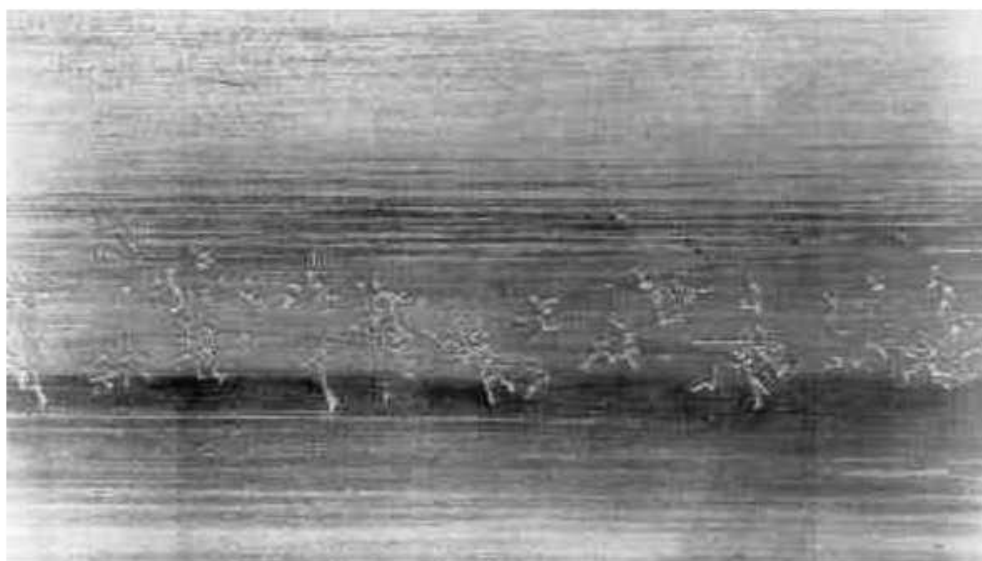
Figure 8 — Cracks in the overlay of a multilayer bearing in a narrow area of high loading (material: steel/lead bronze/electroplated overlay)
