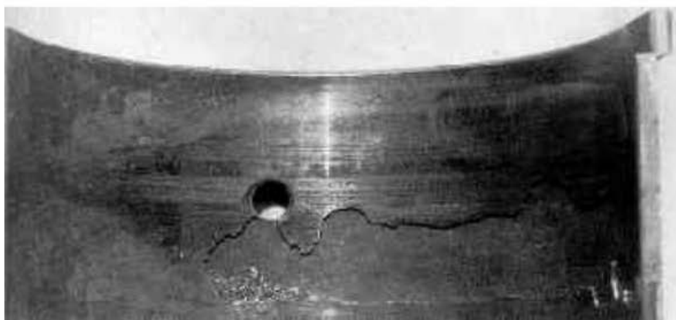
Figure 50 — Loss of white metal showing a break with clearly defined borders (material: steel/tin-based white metal)
