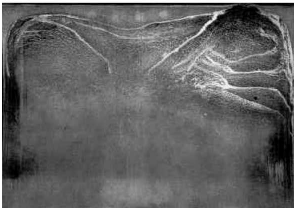
Figure 3 — Creep deformation, shown by crack-free semicircular bulges in the direction of rotation (material: steel/tin-based white metal)
