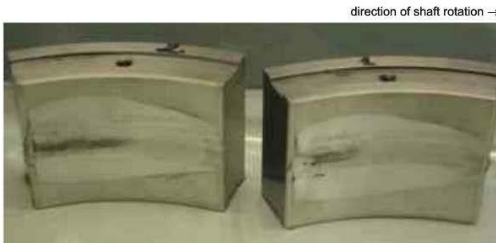
Figure 18 — Creep deformation due to overheating with formation of black depositions (material: steel/tin-based white metal)
