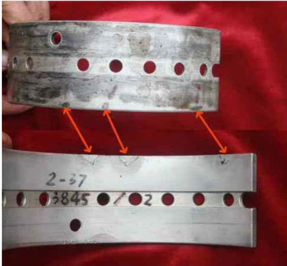
Figure 11 — Material relief by dynamic overload because of insufficient fit on the bearing back (see also 7.2)
