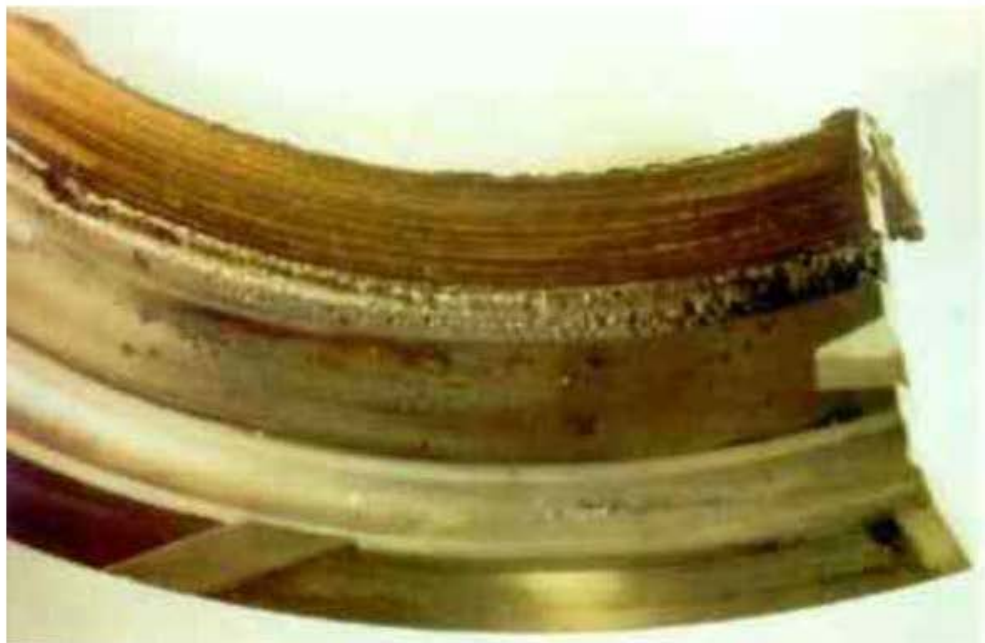
Figure 26 — Melting at the bearing edge and within the groove (material: steel/lead bronze/electroplated overlay)
