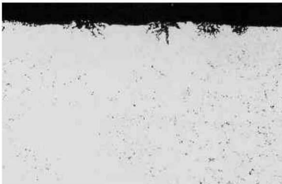
Figure 40 — Corrosion of the surface layer with selective attack on copper and lead in a tin-based material, unetched (material: steel/tin-based white metal)
