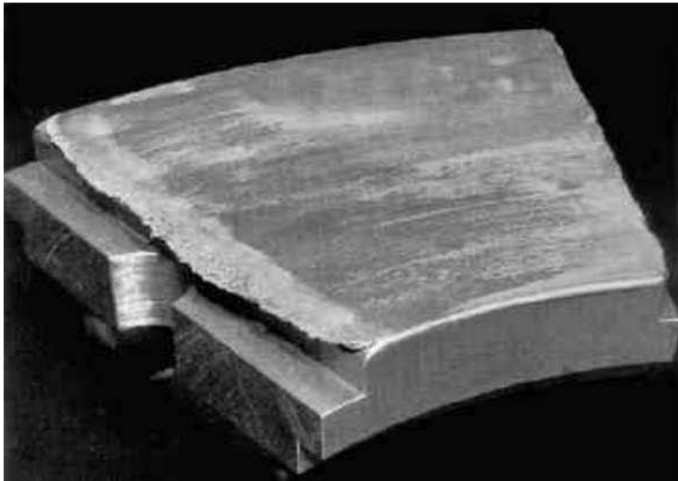
Figure 16 — Wear by friction due to segment assembling on different levels — worn material from one segment deposited on the leading edge of the next segment in the direction of rotation — the segment shown gets a reduction in oil supply (secondary damage characteristic: loss of lubricant) (material: steel/tin-based white metal)
