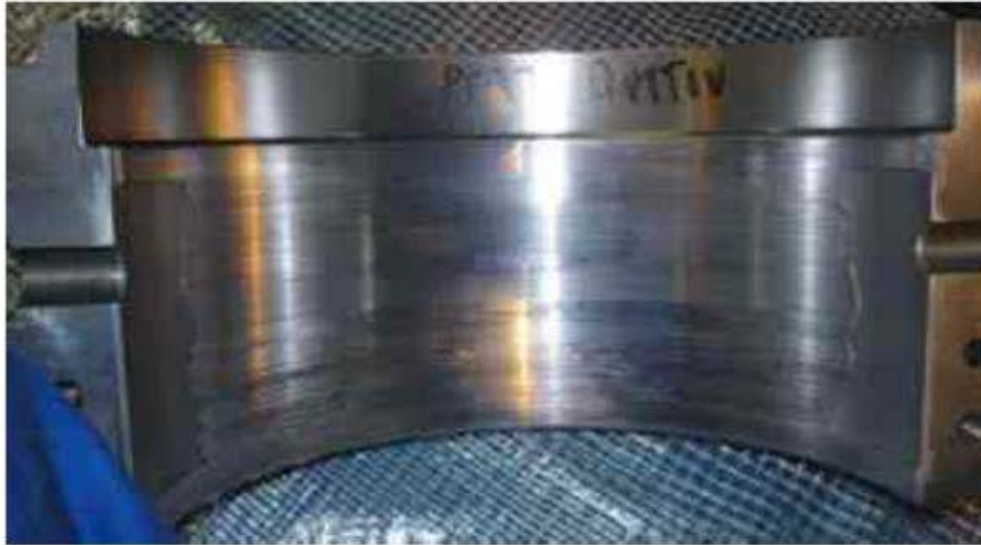
Figure 4 — Propeller shaft bearing, showing the effects of too slow a speed in relation to load capacity (material: steel/tin-based white metal)
