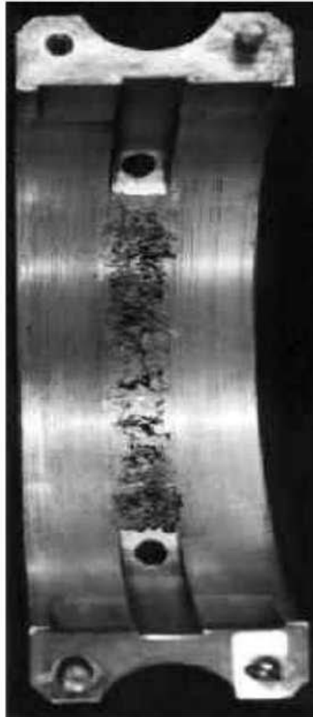
Figure 43 — Typical cavitation erosion on a thick-walled bearing (material: steel/tin-based white metal)
