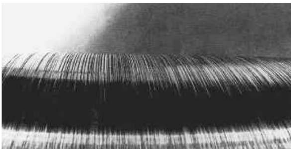
b) wire wool on the shaft
