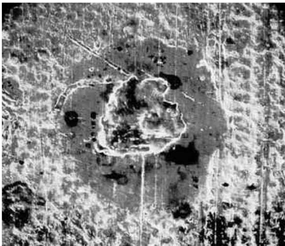
Figure 30 — Crater left by displaced particle surrounded by reflective ring (halo), characteristic of embedding, see Figure 28, label 6, (material: steel/lead bronze/electroplated overlay)
