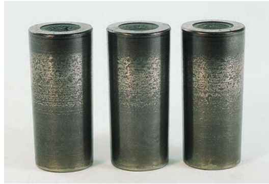
Figure 31 — Indentations from particles on tapered rollers
