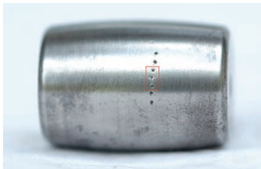
Figure 21 — Roller of a spherical roller bearing — Craters formed by the passage of excessive electric current
