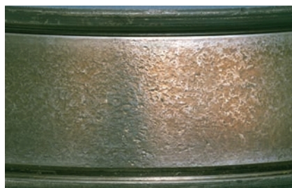
Figure 30 — Indentations from particles on the inner ring raceway of a tapered roller bearing
