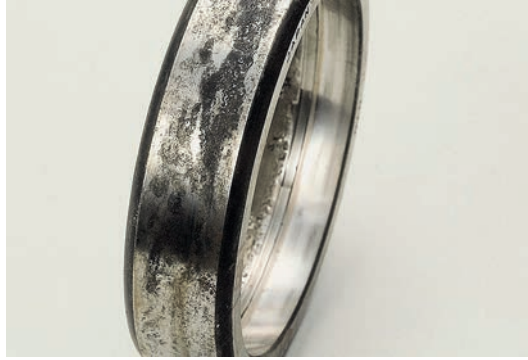
Figure 18 — Fretting corrosion on the outer diameter of a roller bearing
