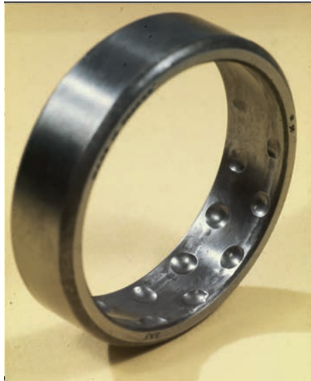
Figure 20 — False brinelling on the outer ring raceway of a self-aligning ball bearing
