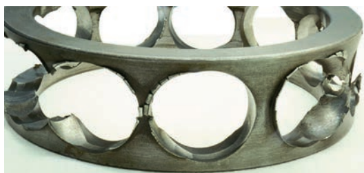
Figure 9 — Advanced abrasive wear on the cage pockets of a solid metal cage
