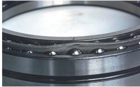
Figure 28 — Cage deformation of an angular contact ball bearing caused by a shock load during handling
