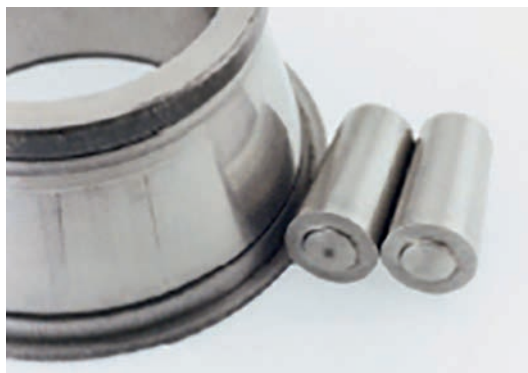
Figure 10 — Abrasive wear on the raceway of the large rib surface of the inner ring and on the large end face of rollers in a tapered roller bearing
