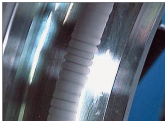
Figure 25 — Fluting on the outer ring raceway of a deep groove ball bearing
