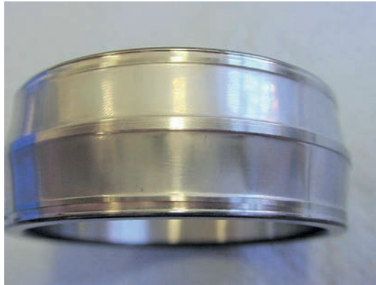
Figure 8 — Abrasive wear on the inner ring of a spherical roller bearing
