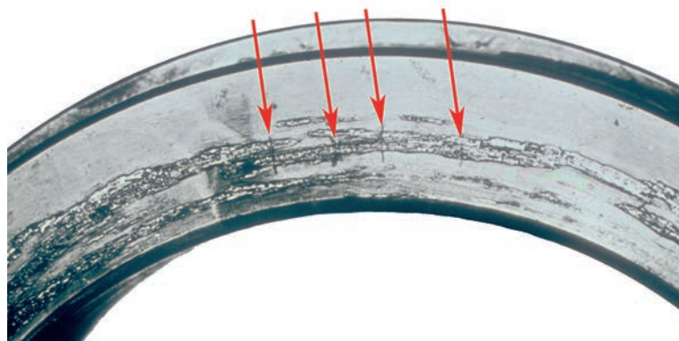
Figure 37 — Thermal cracks on the small end of the inner ring of a tapered roller bearing
