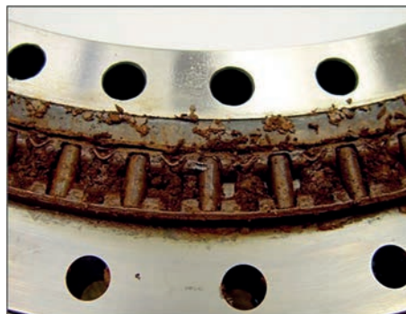
Figure 14 — Moisture corrosion on the cage and rollers of a needle roller thrust bearing
