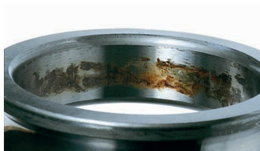
Figure 17 — Fretting corrosion in the inner ring bore of a deep groove ball bearing
